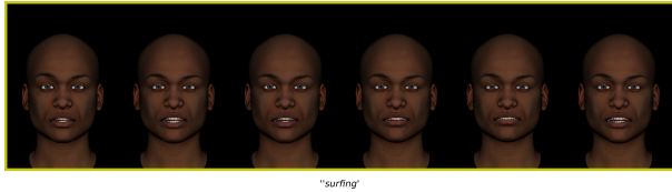
Figure 7: Generated frames given the input phonemes sequence "surfing". We can notice the bottom lip raises up to the bottom of the top teeth to generate the viseme "f".
